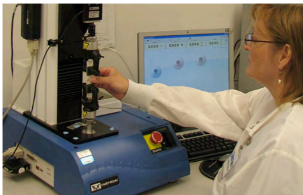
Adhesion Strength Method is used to determine the adhesion strength of a bond between similar or dissimilar materials.
