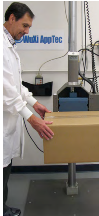
Drop testing of loaded boxes by the free-fall method.
