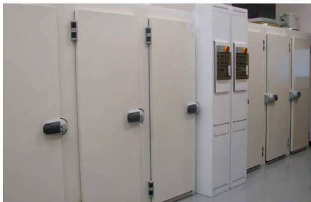
Environmental chambers at WuXi AppTec used for accelerated aging offer a range of temperature and relative humidity settings for conducting package stability performance testing.
